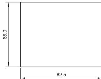
Figure 1-5 Mounting Hole Dimensions of External Operation Panel
